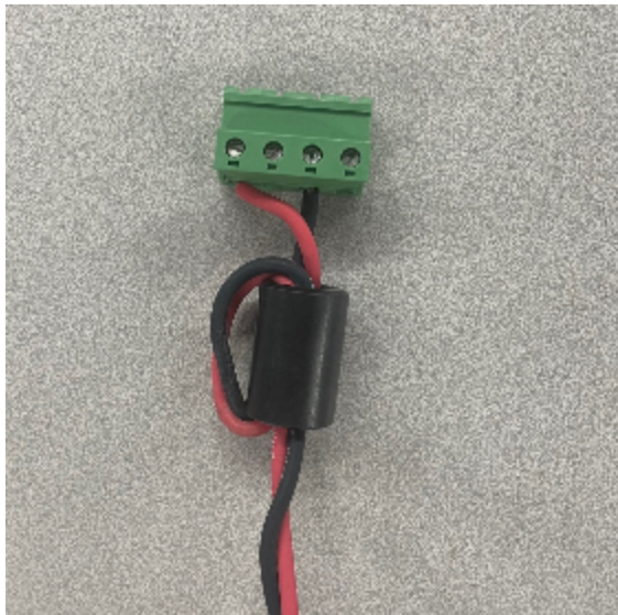
Sample setup for DP5733A model. Provided core and number of turns will vary based on Model Number.
